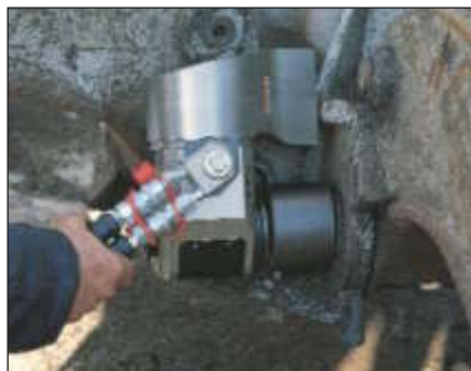
◀ The ZU4 torque wrench pumps are perfectly matched for this SQD-100-I wrench.
